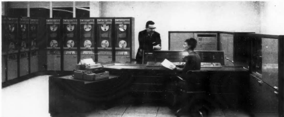
PHILCO 2000 is first large scale all-transistor computer system that has advantage of asynchronous operation—the ability to progress from one operation to another almost
